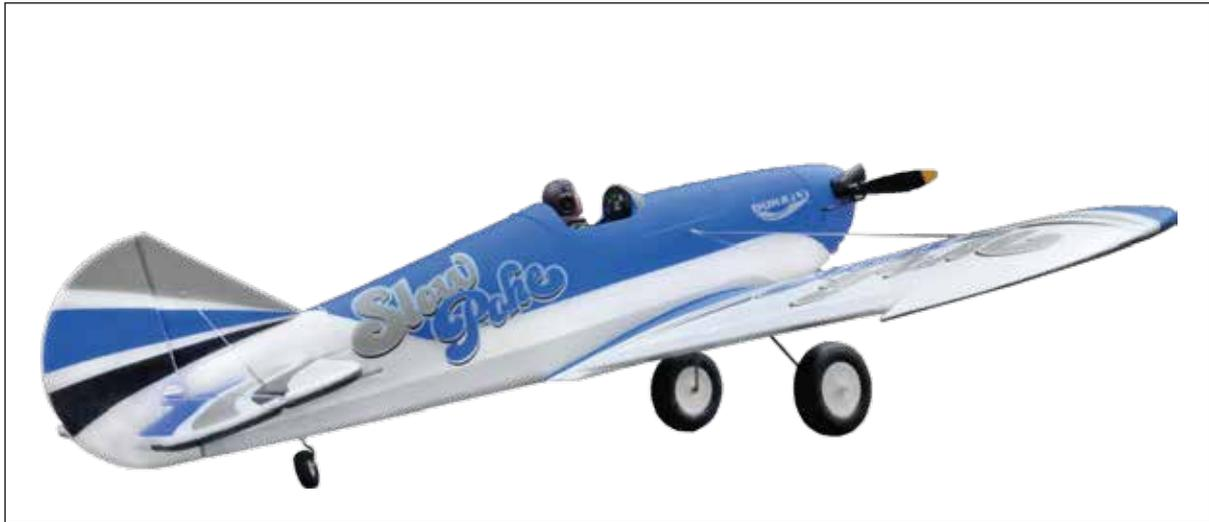
The center gravity(CG) for the Slowpoke is approximately 85-88mm from the leading edge of the wing.
