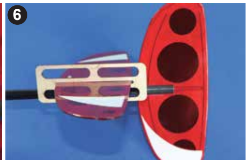
Slide on the provided wooden jig to hold the elevator in straight and level for servo linkage setup.
