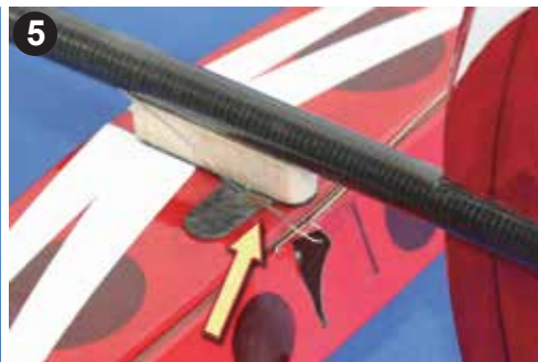
Hook up the prepared cable to the elevator horn as shown.
