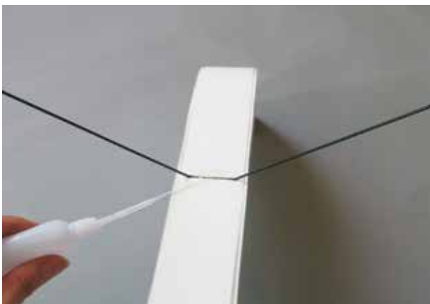
5. Insert the landing gear and landing gear plate into the landing gear slot in the fuselage and use thin CA glue to secure.
