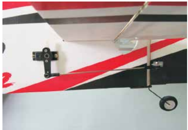
28. Setup the rudder linkages as shown.
