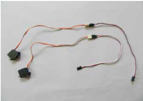
1. Connect servo extension leads to the elevator and rudder servo cables.
