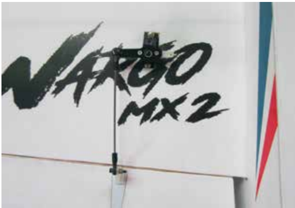
29. Setup the aileron linkages as shown.
