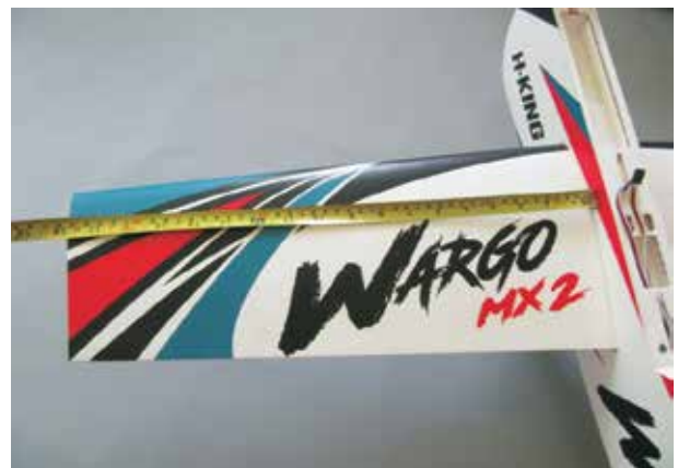
6. Carefully insert the wing into the fuselage. Measure to ensure that both front and rear of the wing are evenly spaced on both sides of the fuselage.
