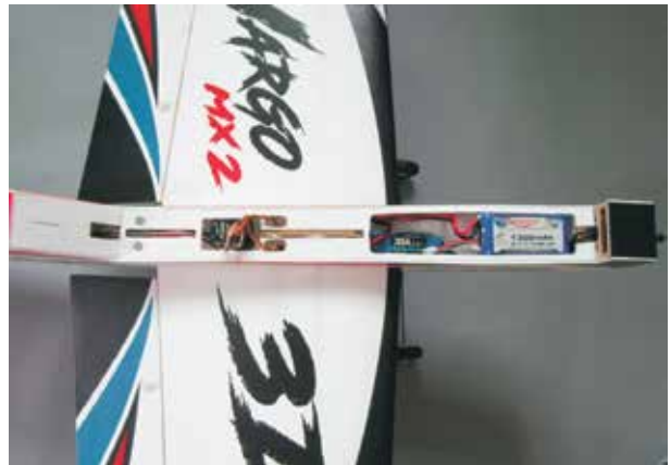
30. Install a receiver. Connect all 4 servos and the ESC to the receiver. Turn on your radio and attach a battery to the ESC. Note: Do not install a prop onto the motor at this moment until all the control surfaces have been well adjusted and ESC has been well calibrated.
