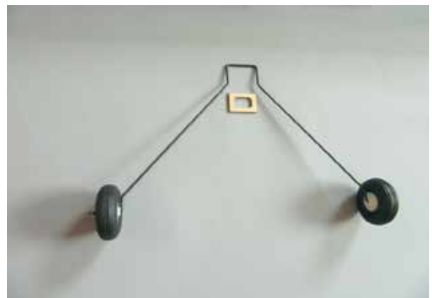
4. Find the landing gear and install the wheels.
