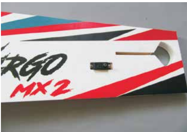
3. Install the rudder elevator and servos into the airframe.
