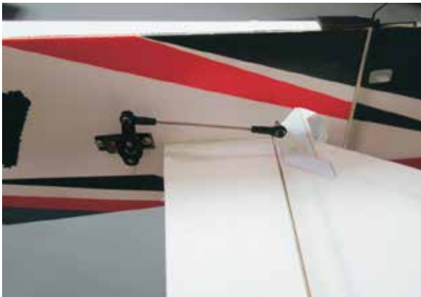
27. Setup the elevator linkages as shown.
